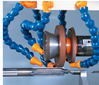
Between-center tooling to grind longer tools on the ETGplus
