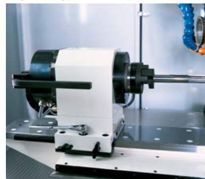
The ETGplus features a movable direct-drive headstock
