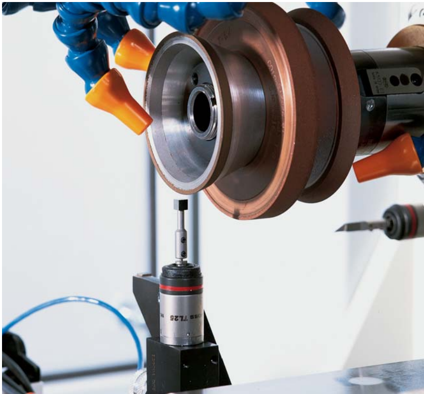
Automatic grinding wheel probing system for ETGplus only
