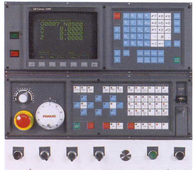
Machine operator's panel with keyboard-type manual data input and 9" CRT color display.
