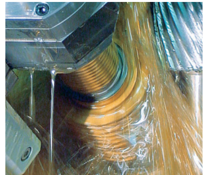
Hob spindle with tools for different gears
