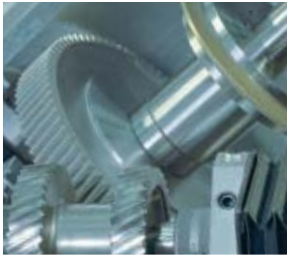
Profile grinding and shave grinding with CBN tools
