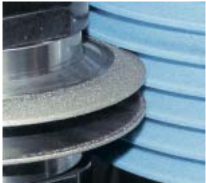
Integrated dressing spindle to adjust pressure angle and tooth thickness of the grinding tool
