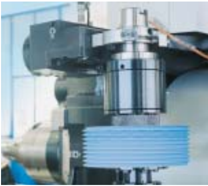
Integrated automatic tool change
