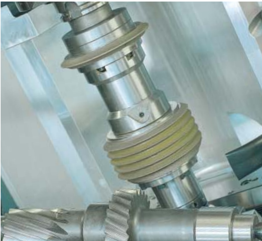
Integrated dressing spindle for flank dressing of the grinding tool
