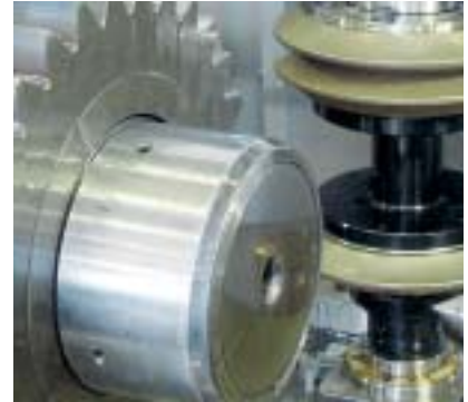
Profile grinding of large module gears with multi-rib CBN grinding wheels.
