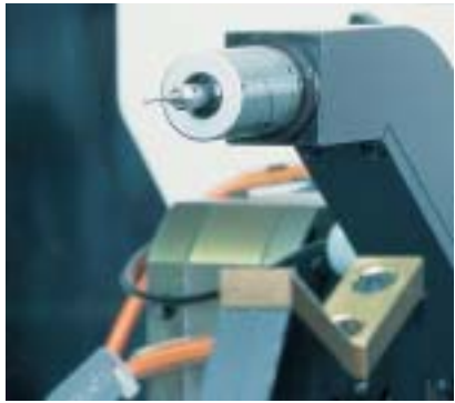
Integrated measuring unit with touch probe
