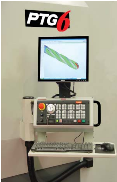
Pivoting operator console
