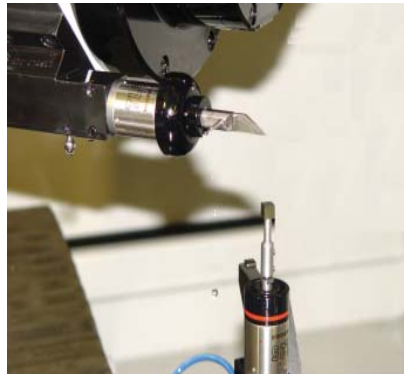
Part Probe on the Grinding Spindle
