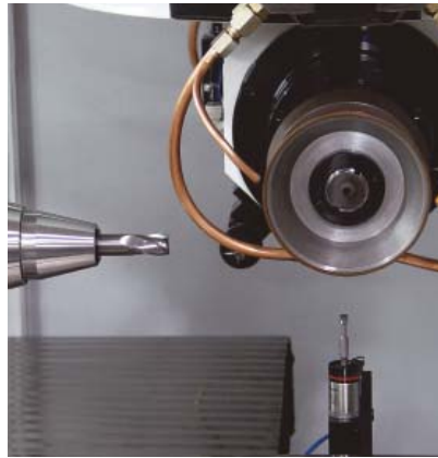
Automatic Grinding Wheel Probing
