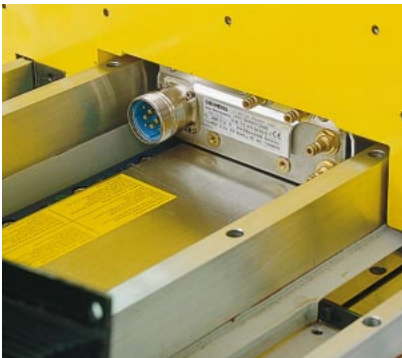
Digital linear motors for all profile-generating axes
