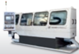
S 3000 GW Ø 400 mm profile depth 52 mm length 3,600 mm horizontal workpiece axis
