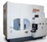
HS 1280-450 Ø 450 mm mn 12.7 face length 300 mm
