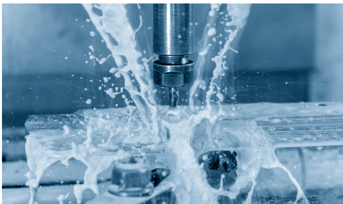
Flood Coolant System
