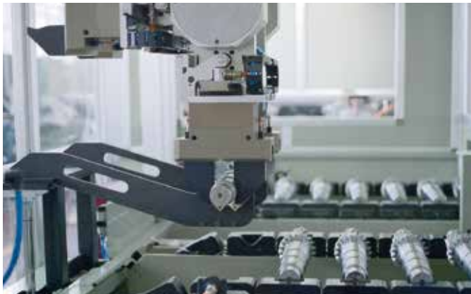
Integrated heavy-duty gantry loader and workpiece conveyor
