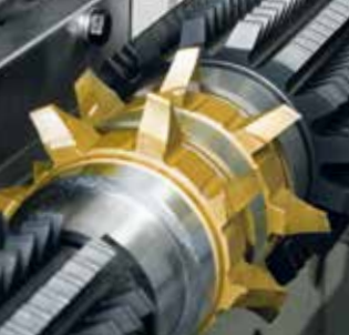
Chamfering/deburring with chamfer hobs
