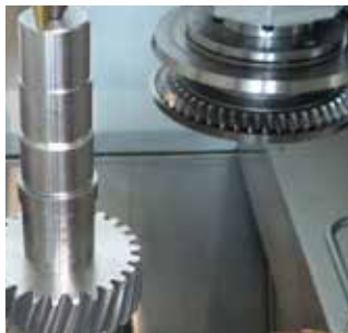
Integrated combination tool for chamfering/deburring on one spindle
