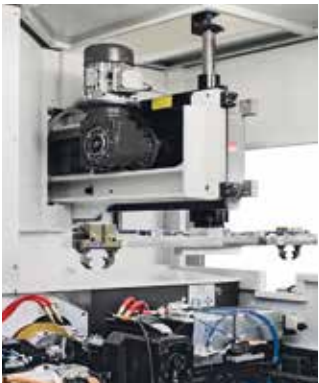
Rotary charger configuration (gantry or robot load as option)
