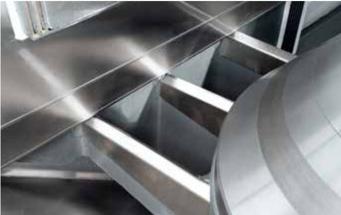
Stainless steel workarea enclosure for dry hobbing
