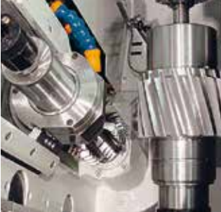
High performance cutting of workpieces with large modules with optimum removal rates
