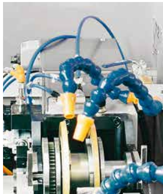
Horizontal workpiece axis for optimum residue fall
