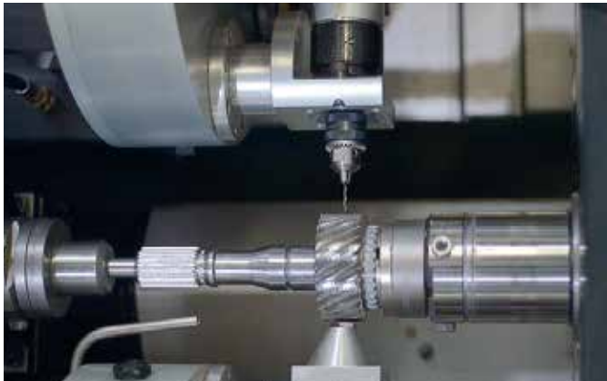
Integrated unit for the drilling of lubrication channels in one setup
