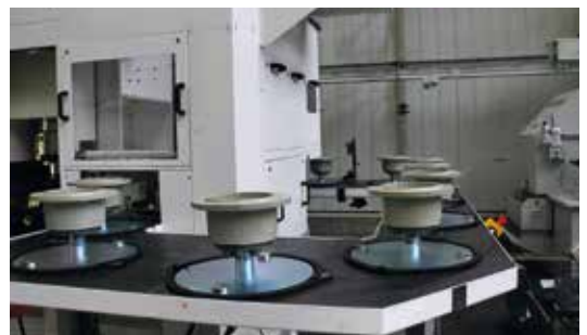
Chain driven conveyor with pallets
