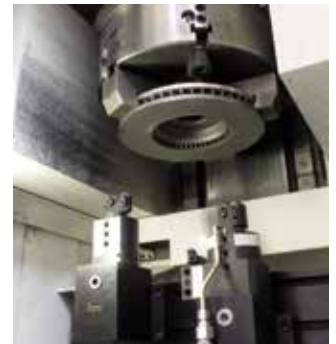
Step 2: Machine 1st side
