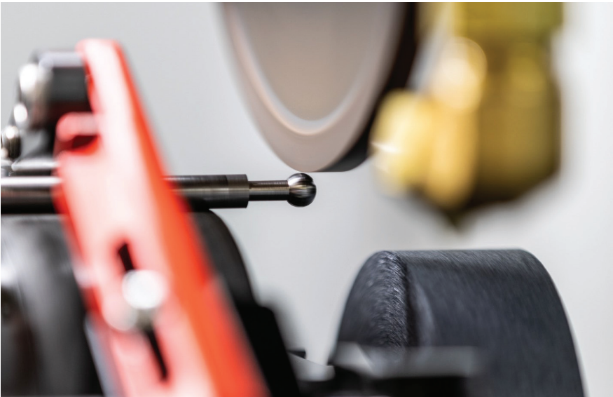
Centerless grinding works with the part being fixtured only on one end while the grinding wheel, or wheels rotate relative to one another to remove material.
