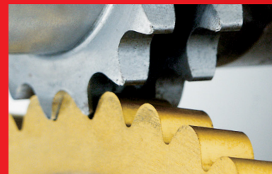
Rolling of a chain sprocket gear.
