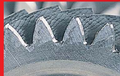
Workpiece after chamfering and deburring.
