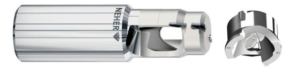
**Solution:** Special PCD designed tool with a 3D printed cage chip deflector steers the cutting chip back into the tool body so that this chip doesn't get left inside the part.
