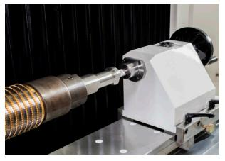
Standard screw actuated tailstock allows for the precise work between centers. Rail mounted, the tailstock can be easily moved to accommodate different setup lengths.
