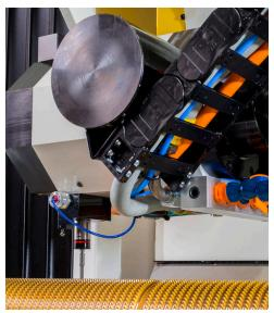
The dual probe system allows for a part probe to locate the cutting edges of the workpiece and reference it to the machine while the wheel probe (shown) locates the grinding wheel relative to the workpiece.
